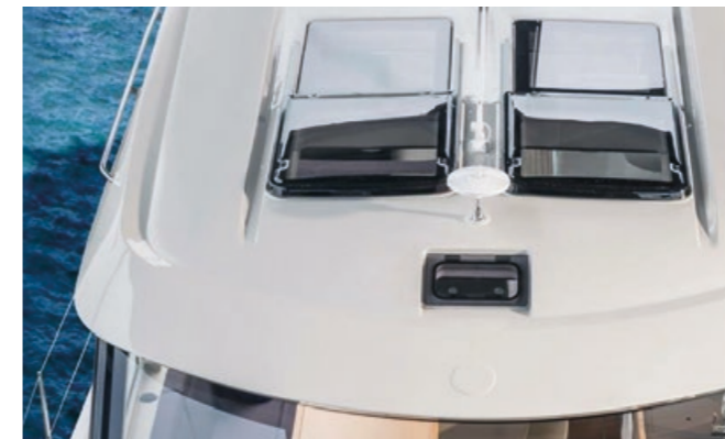
Innovative light weight electrical sliding roof
