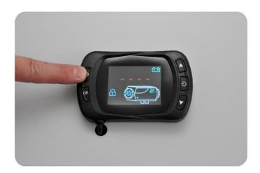
**Heater ambient temperature**. Press **ok** button once to see the ambient temperature at the heater.
