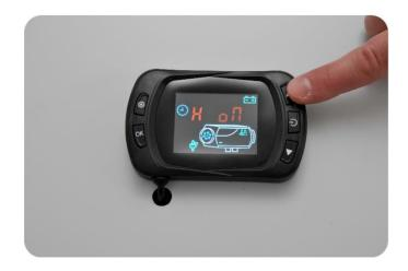
**3.3 Turn Off**. To deactivate the fuel pump press the **down** arrow.
