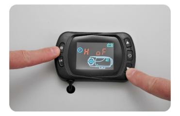
**Turn On**. To activate the fuel pump press the **up** arrow.
