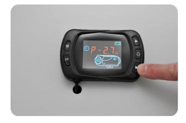
**5.2.3** Lower Temperature. Press the down arrow to lower the temperature.
