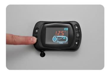
**Altitude**. Press the **ok** button four times to see altitude. Note: Altitude is factory set and can't be changed by the user.
